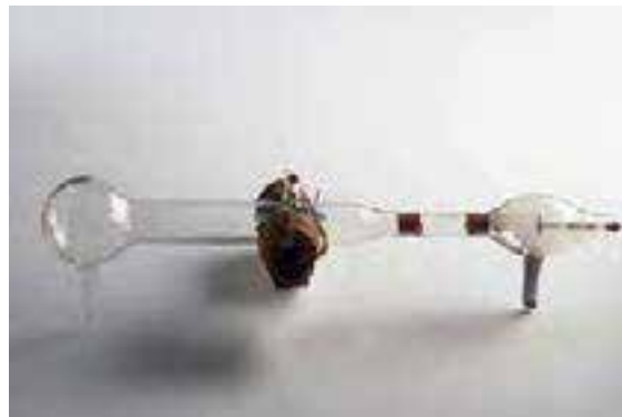
Fig. 2.1: J. J. Thomson's cathode-ray tube that he used for the discovery of the electron.
