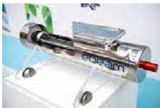
Fig. 4.13: Tetra Pak has a new generation of automated filling machines that uses e-beams to sterilise packaging.
