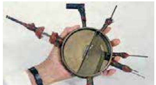
Fig. 2.4: The Lawrence and Livingston cyclotron. This was 13 cm in diameter and accelerated a proton beam to 80 keV.
