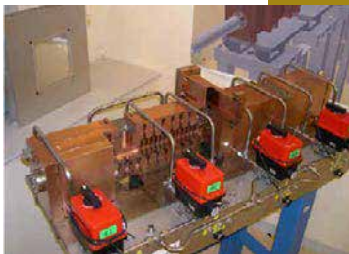
Fig. 3.8: The TERA side-coupled linac structures (shown) and other, later high-gradient structures have been proposed for a variety of particle-therapy applications, including proton and carbon-ion treatment, and the delivery of very high-energy protons for imaging and novel treatments (credit: Adriano Garonna/TERA Foundation).
