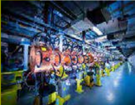
Fig. 2.3: The linac at CERN used to prepare proton beams for the Large Hadron Collider.
