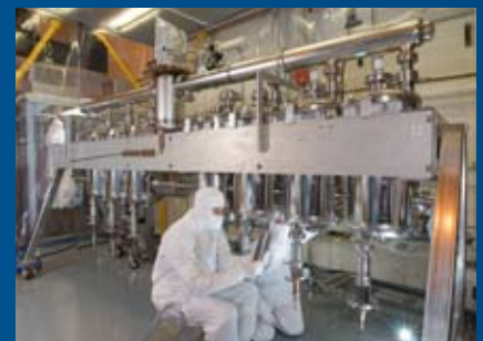
Assembly of a superconducting accelerator section for production of ion beams Photo courtesy of J. Nolen, Argonne National Laboratory
